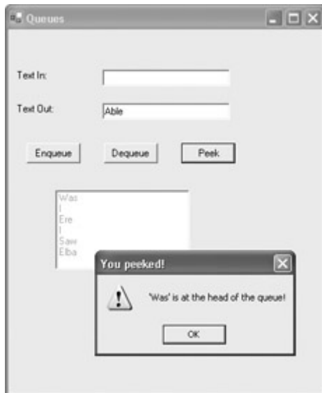
Figure 7.8: With 'Able' dequeued, peeking discloses that 'Was' is at the front of the queue.
