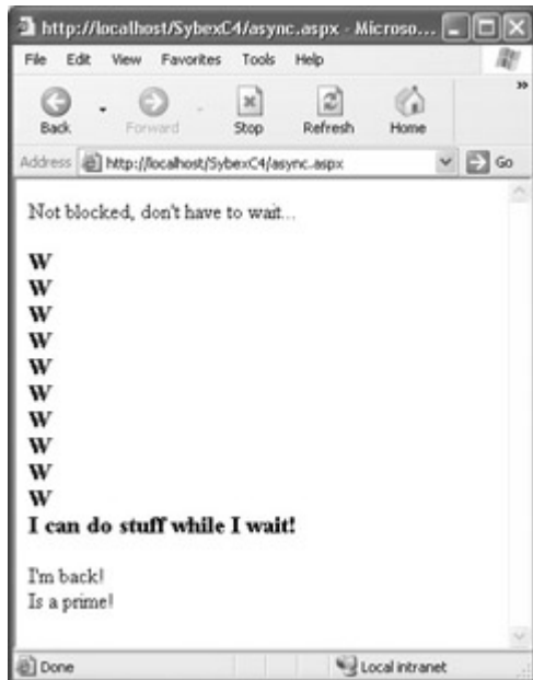
Figure 2.18: The W s are written one after another to the screen, then the asynchronous call completes.
