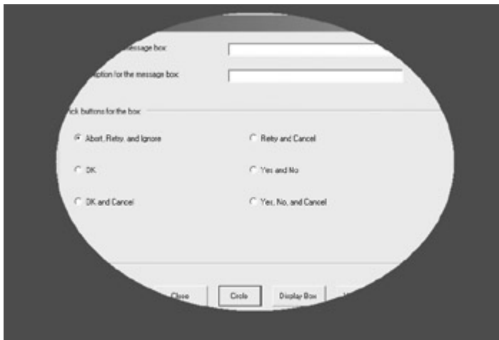
Figure 3.15: The Region property of the form can be used to make it any shape you'd like. Warning Depending on the shape you choose for your form, it may not have the normal mechanisms for closure, as in the example here, because the top part of form has been eliminated. Make sure that you provide a way to close the form (such as a Close button).
