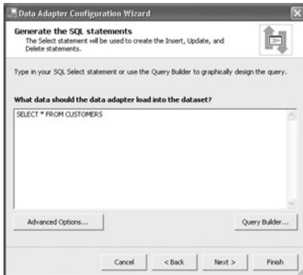
Figure 12.27: An SQL statement is used to determine which data will be used to create the dataset.
