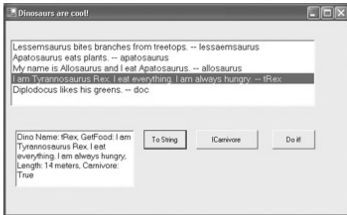
Figure 9.5: It's up to you to implement a meaningful ToString method for your classes (the ToString return value for a TRex instance is shown).
