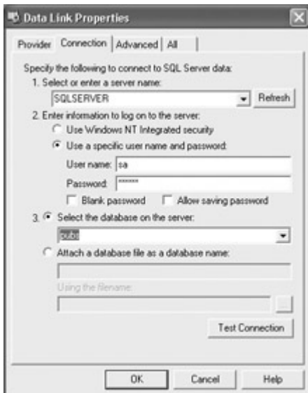
Figure 12.25: The Data Link Properties dialog allows you to create a new data connection.
