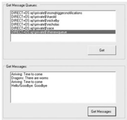
Figure 11.13: You can use an array of messages to retrieve the subject and text of all messages in a queue.
