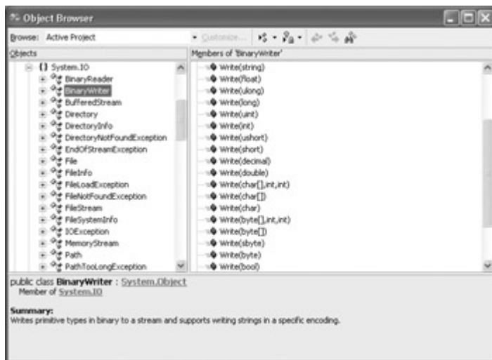
Figure 10.10: The overloaded variants of the BinaryWriter.Write method allow you to easily write a variety of primitive types to a binary file.
