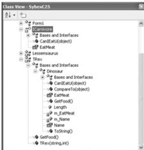
Figure 9.9: The ICarnivore interface (and the members of the TRex class) are shown in Class View.
