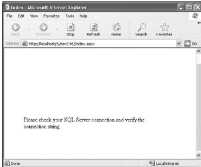
Figure 13.15: It's important to include exception handling in the client application if the web service involves database connectivity.
