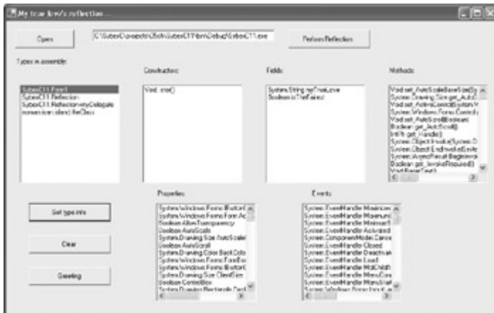
Figure 5.7: Variables declared at the form's class level appear as Fields; all form methods, properties, and events are displayed in the appropriate ListBoxes.
