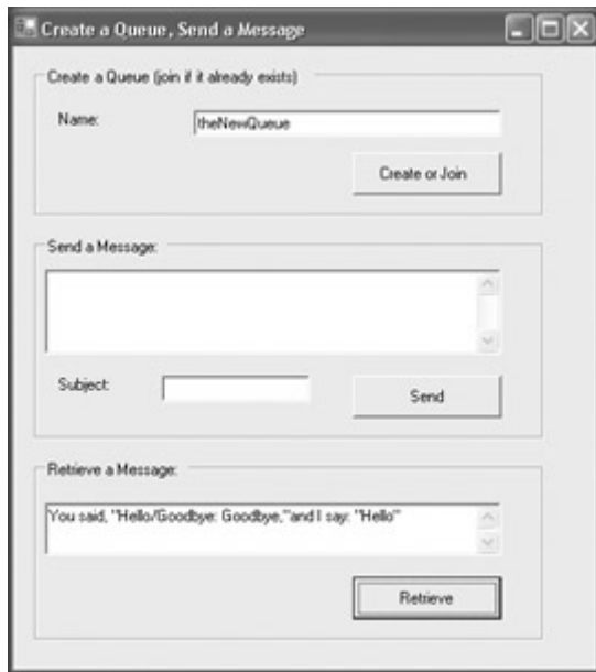
Figure 11.15: The Receive method takes the first message off the queue, regardless of what program sent it.
