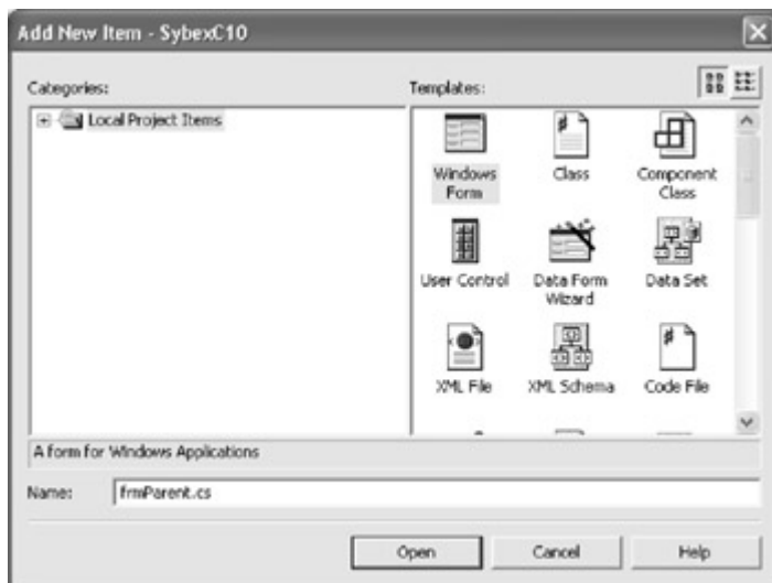
Figure 4.16: The Add New Item dialog is used to add a 'parent' form to a project.
