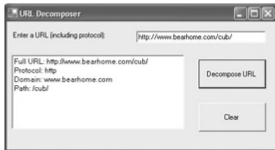
Figure 9.14: Regular expressions can be used to decompose a URL into constituent parts.
