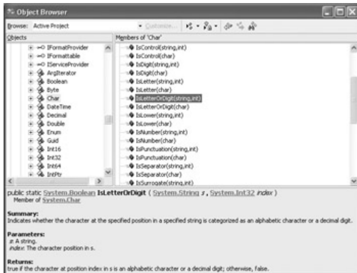
Figure 9.1: The static methods of the Char class-shown here in the Object Browser- allow discovery of the nature of individual characters.
