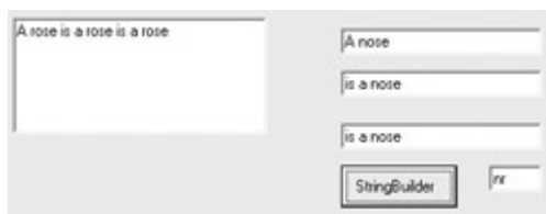
Figure 9.4: The StringBuilder Replace method can be used to replace all instances of a character in a StringBuilder with another character.
