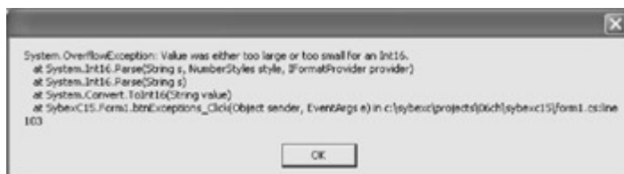
Figure 6.9: The ToString method of the Exception object contains a great deal of information about a thrown exception.
