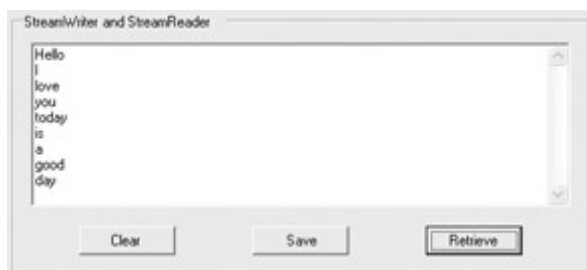
Figure 10.8: The StreamReader reads the text in the selected file into the multiline TextBox . Listing 10.8: Using a StreamReader to Retrieve Text
