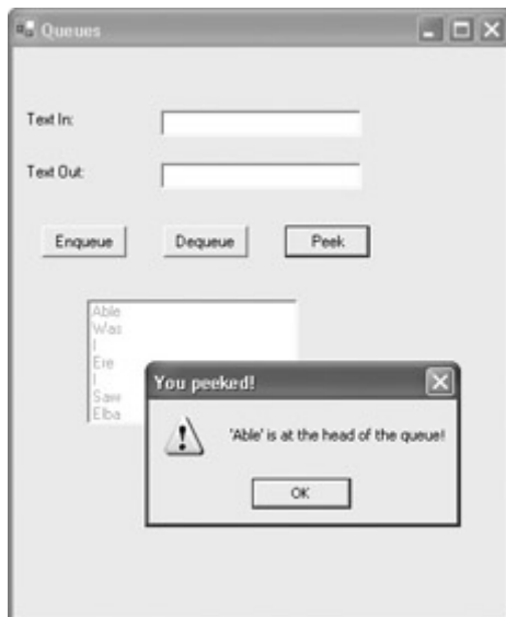
Figure 7.7: Peeking retrieves the object at the front of the queue without removing it from the queue.
