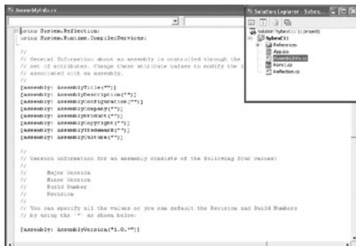
Figure 5.1: Each C# .NET project includes a file that forms the basis of the assembly manifest. The manifest carries information about content, version, and dependencies so that C# .NET applications don't depend on Registry values.
