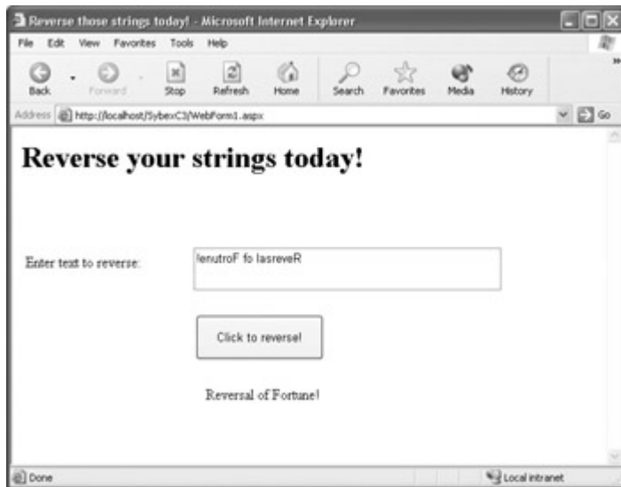
Figure 2.12: The application invokes the web service in the code-behind module to reverse the string.
