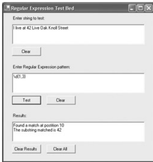
Figure 9.12: It's easy to set up a program that can be used to test regular expressions.
