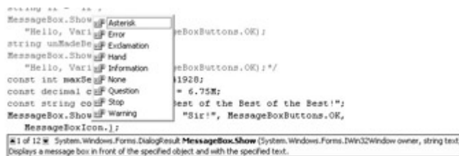
Figure 6.1: The auto-completion feature of the Code Editor supplies the members of an enumerator list.
